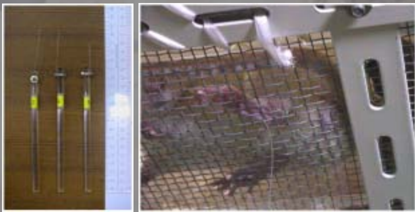
Fig. 1. Method to apply mechanical stimulation. Von Frey hairs were used to apply mechanical stimulation to the plantar surface of the hindpaw. Left: von Frey hairs. Each hair was calibrated to give constant force (from left to right, 34.0, 53.9 and 126.7 mN). In this experiment, we used 53.9 mN force, which does not cause pain sensation when applied to the experimenter. Right: a figure of von Frey hair test. The von Frey hair was applied to the plantar surface of the rat's left (treated) hindpaw.
